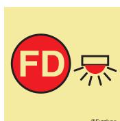
S 10 06 Space protected by automatic fire alarm
